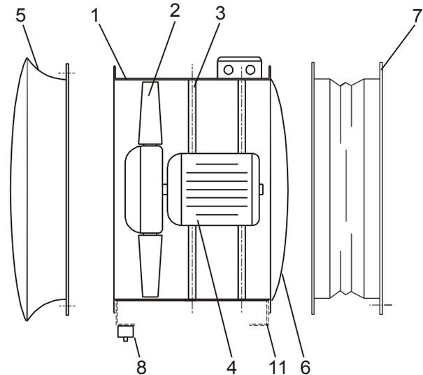
In normal circumstances the fan is built into a ducting system. It can, however, be integrated into a box in order to suppress noise, which is then built into the ducting system.
